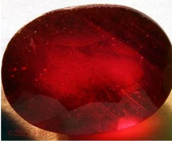
Glass filling is easily visible with 10x loupe. The surface will have a “cracked glass” appearance as seen below left, with large gas bubbles being visible under magnification as seen below right..
